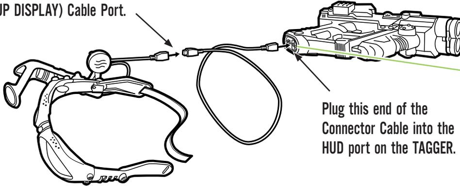
Plug this end of the Connector Cable into the HUD port on the TAGGER.
