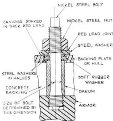
Typical armor bolt used for securing the Class A upper belt to its STS backing plate. One bolt per every 5 square feet of armor plate.
