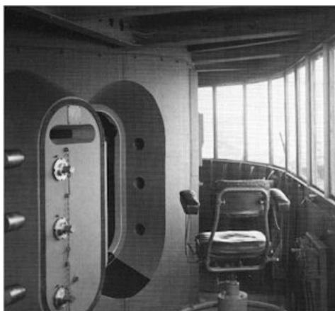
The interior of the ship's bridge. At 17.3 inches, the conning tower armor is among the thickest in the ship. Notice the viewing slit in the door.
